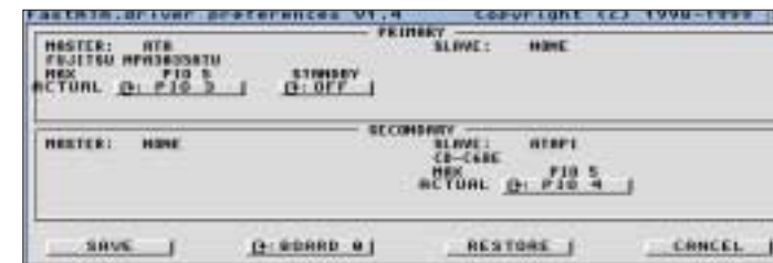
Above: FastATAPrefs showing a hard drive on the first port and a CD-ROM on the second.
