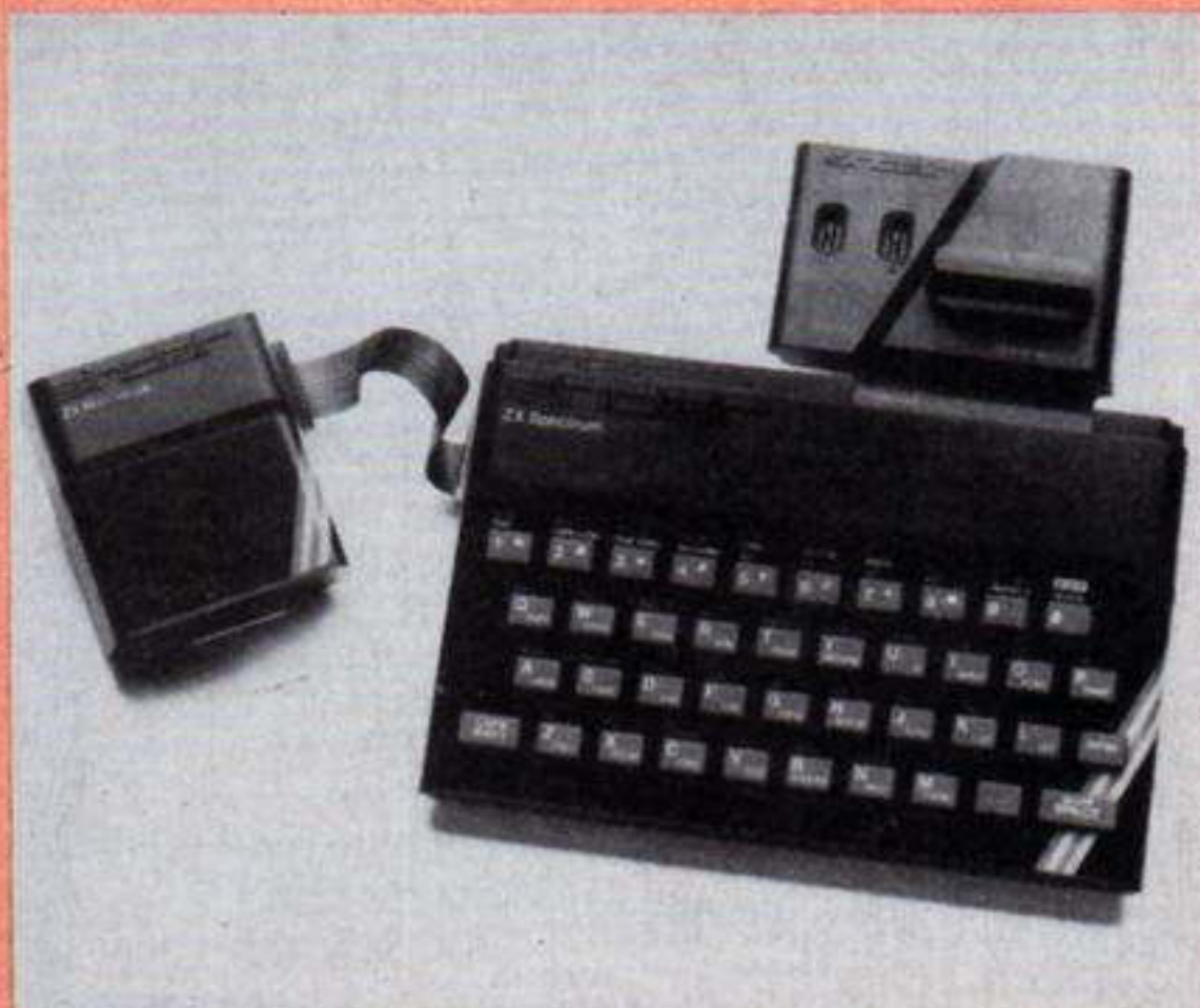
The Interface 2 plugged into the Interface 1. Nice sockets, shame about the shape
