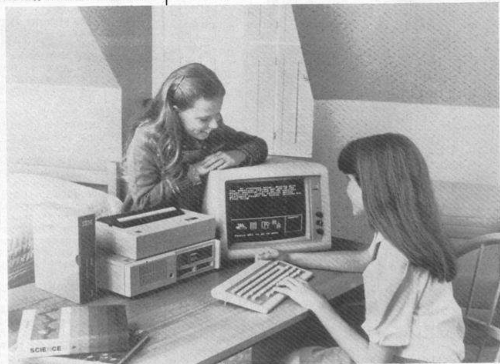
IBM's PC Junior with the thermal printer perched on top of the main unit
